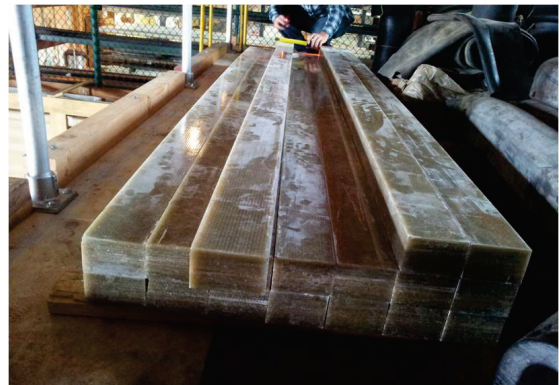
FRP composite miter blocks awaiting installation
