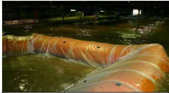
Wave testing of perimeter barrier
