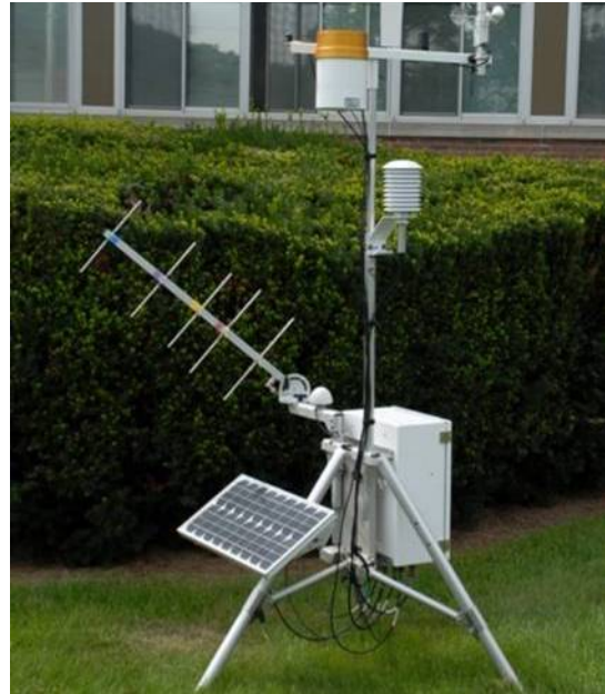
Figure 1. Rapidly deployable flood monitoring system designed to be portable, easily transported/shipped and deployed with minimal effort. Redundant satellite communication systems and a direct link to CWMS allow near real-time web-based access to critical flood information in emergency situations.
