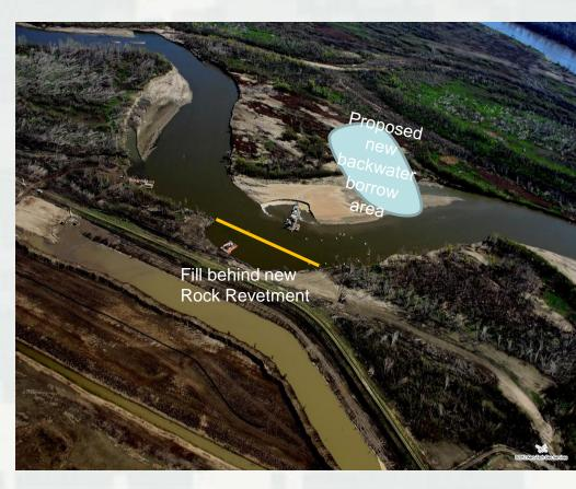
BLUF: Dredging of backwater for shallow water habitat provides fill for repair at less cost as other sources while supporting habitat creation for the MRRP
